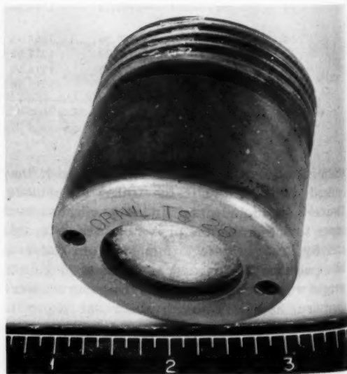
Fig. V-5 Teletherapy source cracked by 84,000-lb force. Note crack through "L" in ORNL. Ruler is marked in inches.
